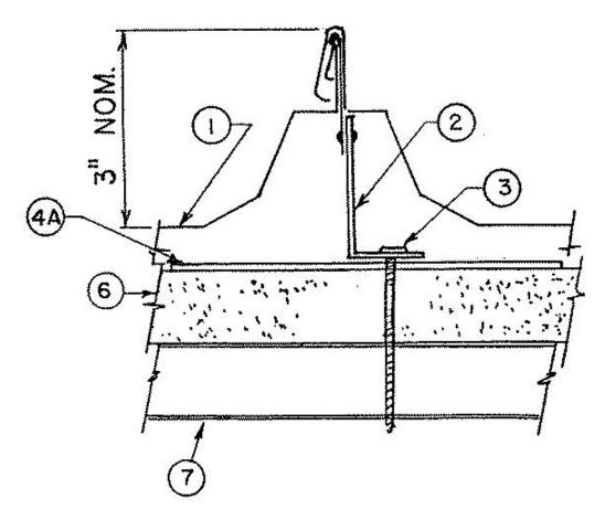
1. Metal Roof Deck Panels\* — 24 MSG min coated steel. Panels continuous over two or more spans. End laps to occur adjacent to purlin with panels overlapped 3 in. A line of sealant may be used at panel ends and side laps.
